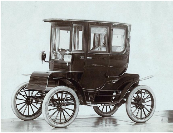
Typical Electric car of the late 1880's, the earlier models usually open with no windscreen, and a folding roof.
