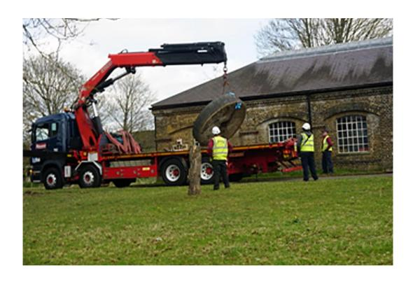
Here you see the lorry that has just arrived from Fort Halstead unloading the mill stone. It arrived late because we had all underestimated the weight of the stone (thought to be four tonnes but in reality nearer six) and the lifting strops had failed when it was being loaded on to the lorry at the Fort. Anyway, it is now back home.
