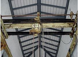
The inside of that building featured a disused overhead crane with a capacity of 5 tons that, once restored, would facilitate maintenance work on Woolwich and Carnegie, the latter shown here on "the Slab" in 2005.
