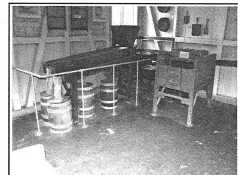
the smallest of our sorting machines in the background and a hand operated corning machine to the right. The sieves on the wall were originally (10 years ago) woven from silk but now of nylon.
