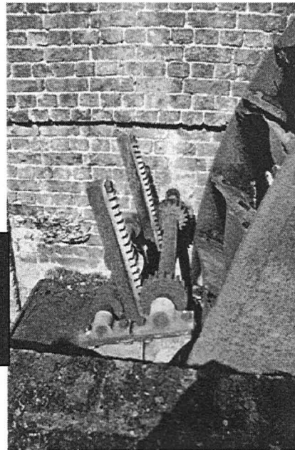
The hatch controls. Note the plummer blocks with the oiling holes set vertically.
