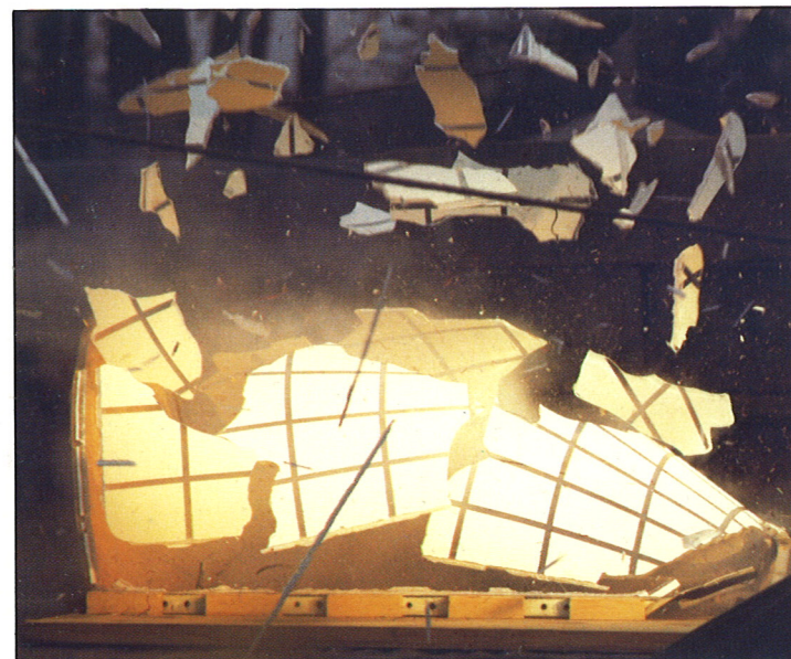
Harrier canopy fragmentation using miniature detonating cord - Fort Halstead.
