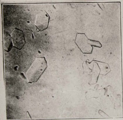
Fig. 3. NITROGLYCERINE IN STABLE, LESS SENSITIVE FORM
