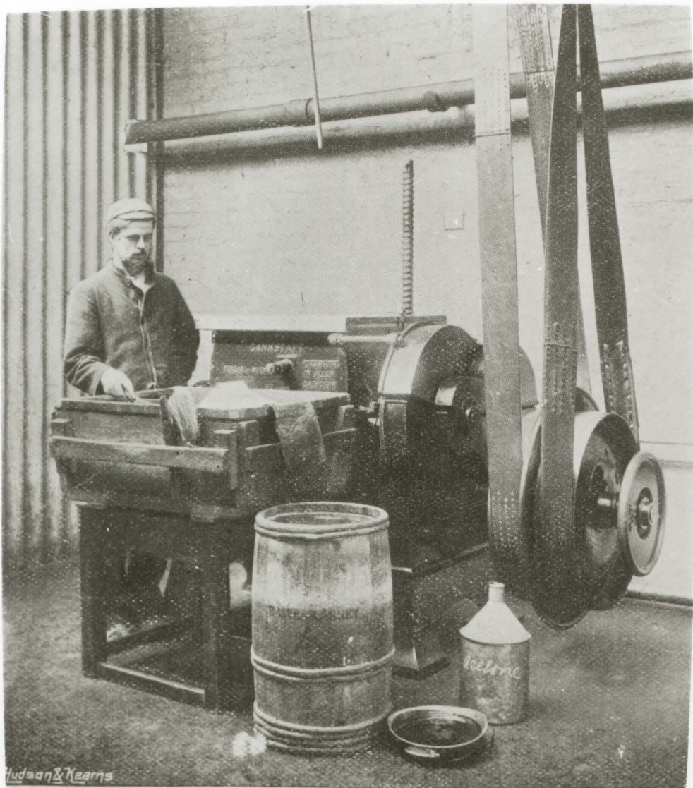
A MACHINE IN ITS TIME PLAYS MAN'S PARTS. Baker's Dough Incorporator Used for Cordite Mixing.
