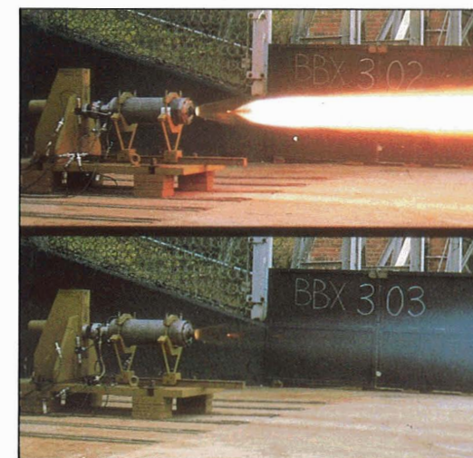
Comparative firing of motors with and without flame suppression additives
