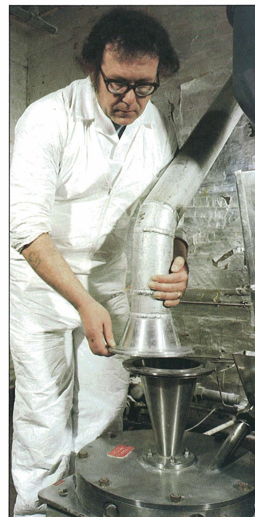
Planetary mixer for composite propellant production. Royal Ordnance has also recently installed a 420 gallon mixer – the largest available in the world today.
