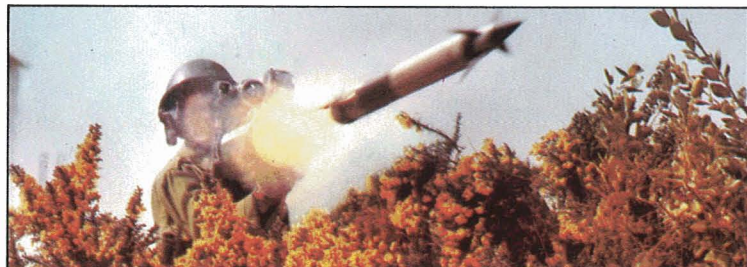
For the operator's safety, the shoulder-launched anti-aircraft Blowpipe missile is fitted with an 'All Burnt On Launch' (ABOL) boost motor, and a delayed-action sustainer
