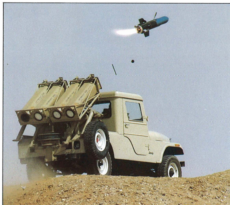
Thrust vector control operating on the Swingfire long-range wire-guided anti-tank weapon
