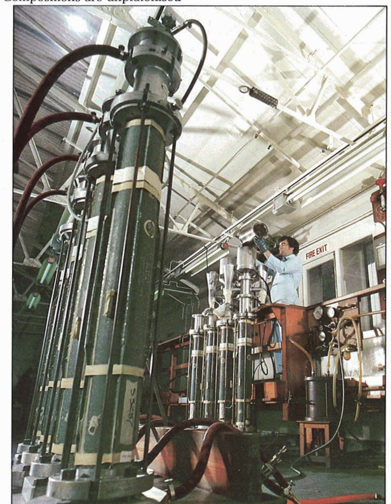
Part of the automated plant for casting propellant charges
