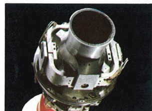
Thrust vector control operating on the Swingfire long-range wire-guided anti-tank weapon
